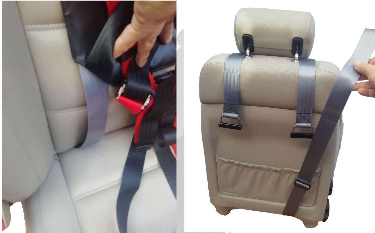
A fixing-strap correctly fed through the gap between the horizontal and vertical parts of the seat.
